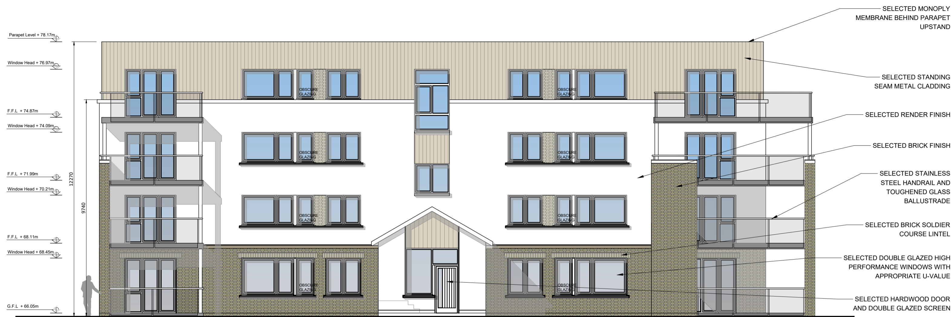
Block C - South-east Elevation
