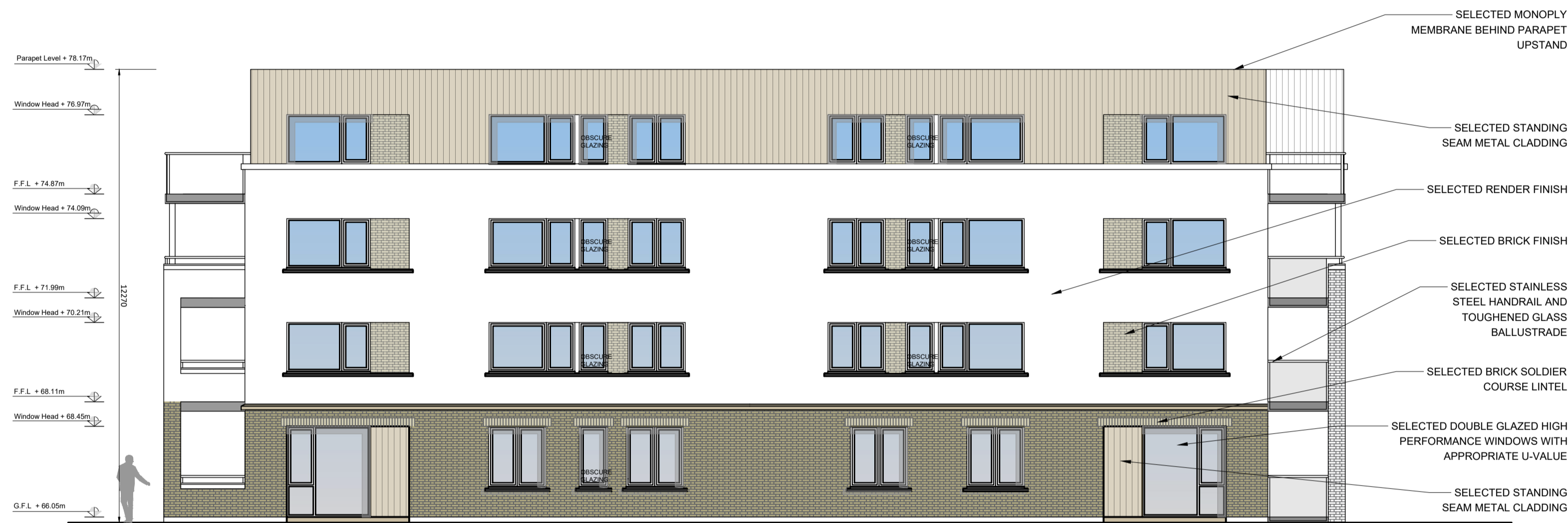
Block C - North-west Elevation
