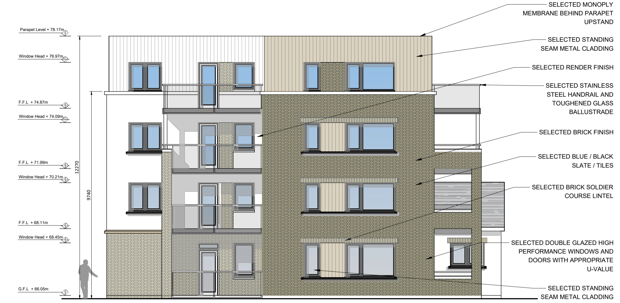
Block C - South-west Elevation
